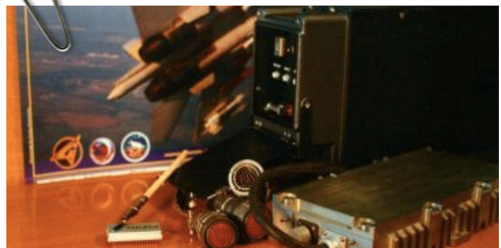
from left to right: new triple memory, active flight control system, flight data recorder all 1994
